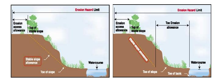
a) Stable toe (floodplain ≥ design toe erosion allowance)
