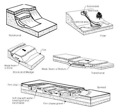
Figure 2 Typical slope movements
